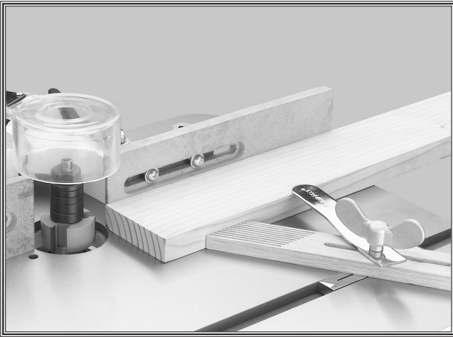
Figure 1. Use a SHOP FOX® Featherboard as anti-kick back protection.
